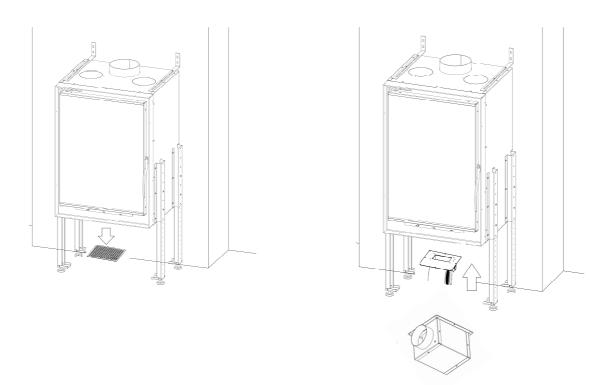
Remove the vent at the bottom of the convection chamber by breaking the micro-couplings.
