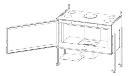
Remove the convection chamber vent by breaking the micro-couplings.
