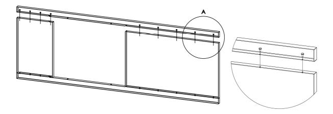
Remove the fireplace door and position and screw the New Line frame to the front of the appliance. Refit the door.
