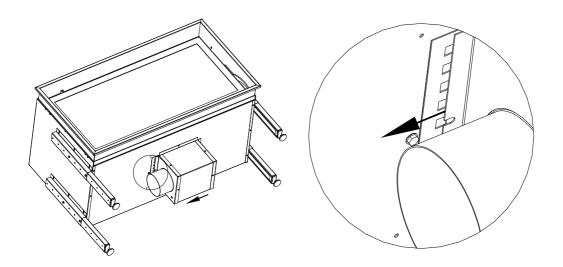
Put the housing down and move it to coincide with the screw tab recess. Then tighten the remaining three screws.
