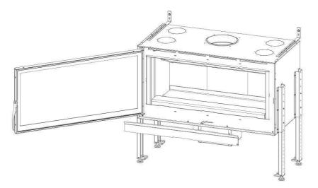
Remove the primary air inlet nozzle
