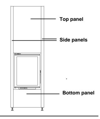
Screw the top and bottom panels to the side panels.
