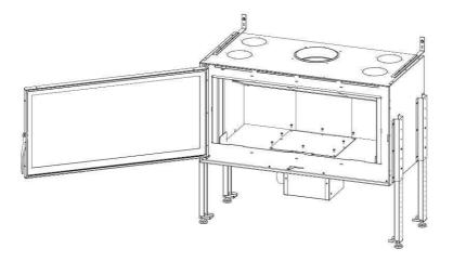
Replace the base, the air inlet nozzle and the woodholder that protects the glass.
