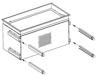
Adjust the height and fasten the legs in place using the screws. To mount the turbine housing, a minimum height of 175 mm is required.
